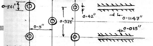
he air flows at a rate of 1500 kg/h perpendicular to the tubes and exits with a mean temperature of 120°C. The core is 0.5 m long with a 0.25 m<sup>2</sup> frontal area. Calculate the total pressure drop between the air inlet and outlet and the average heat transfer coefficient on the air side. Take air densities at the inlet (25°C) and outlet temperature (120°C) from properties table.
